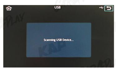
2. Connect USB to the KPLAY board with the update file. The USB media will be scanned automatically
